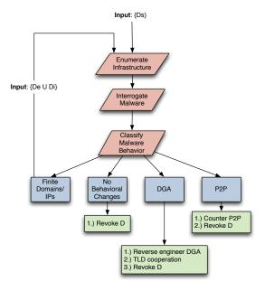
Figure 3: Takedown recommendation engine shown as a decision tree. D in this case represents either  $D_r \cup D_i$ , which only targets C&C domains that are very likely to be malicious or  $D_e \cup D_i$ , or the "nuclear" option that should only be used when the threat of the botnet outweighs potential collateral damage.
